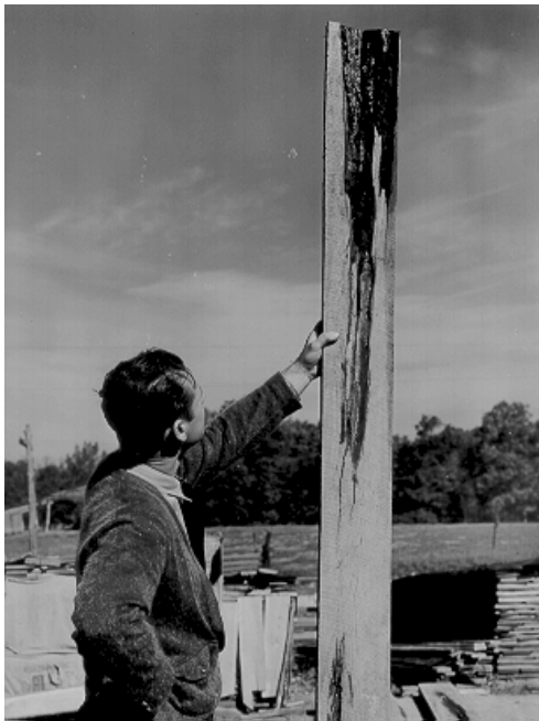
Here an instructor demonstrates the quality of boards sawn from a fire-damaged red oak at a mill near Tell City, Indiana.
